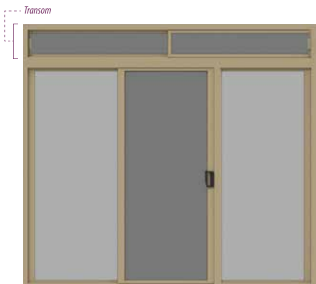
Triple panel center sliding patio door with glass, screen & transom Widths from 96" to 124" | Door heights from 78" to 88" Overall panel heights including Transom up to 120" Transom height with fixed glass 10" to 32" Transom height with sliding glass 14" to 32"
